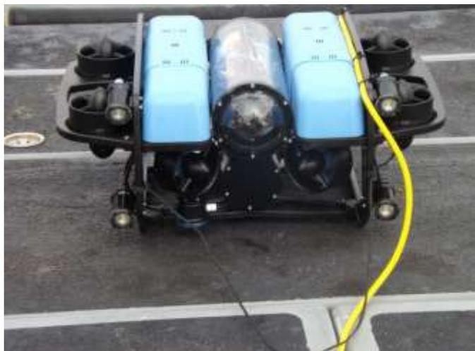
control to be able to steer the BlueROV 2 around a string of pots, and manoeuvrability to allow careful examination of rugged chalk to investigate whether there is any evidence of damage. By continuing surveys with the ROV during neap tides over the coming months, Eastern IFCA will be able to build an up-to-date and robust base of evidence to best inform our management decisions.
