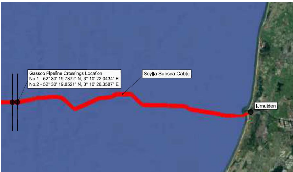
Figure 1. Gassco asset crossing locations in relation to the Scylla subsea cable route (Map image c/o MDM).
