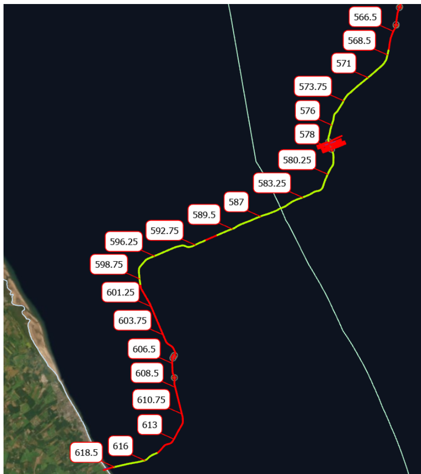
Figure 2: Subsea rock installation in C1 campaign (green lines)
