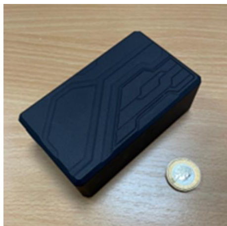
Image 3 Magnetic tracker used by volunteer fishermen to monitor position, speed and direction. £1 coin for scale.
