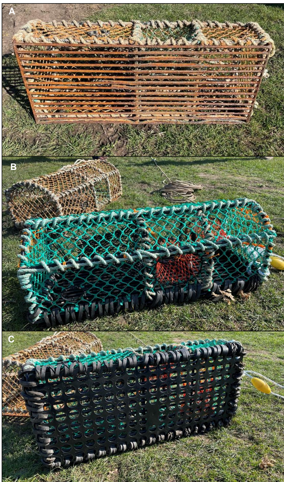
Image 4 A standard parlour pot, viewed from underside (A). A soft-armoured pot (foreground) with rubber banding around frame compared to standard pot (background) (B) and a plastic base (C).
