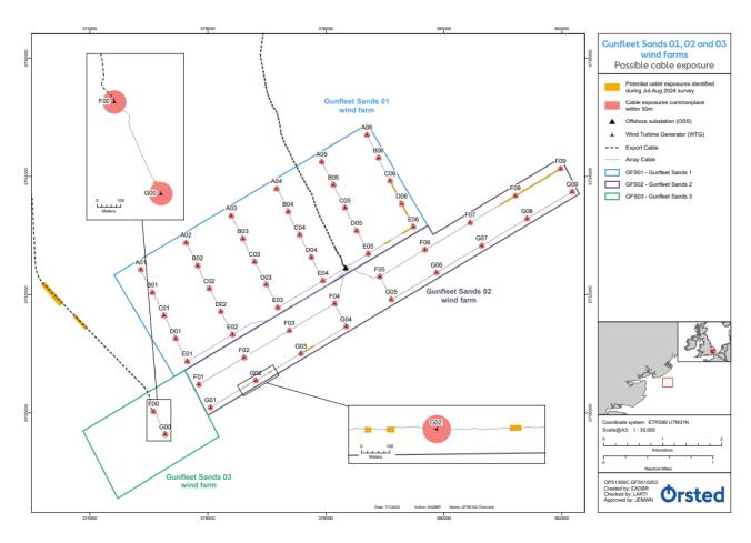
As a result of a sedimentary surface and above average flow velocities, bathymetry within the Gunfleet Sands array area is constantly evolving.
