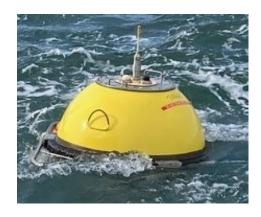
The Waverider Buoy is fitted with a yellow light exhibiting the sequence FI Y (5) 20s. The LED flashlight gives 5 flashes in 10 seconds and repeats this every 20 seconds.
