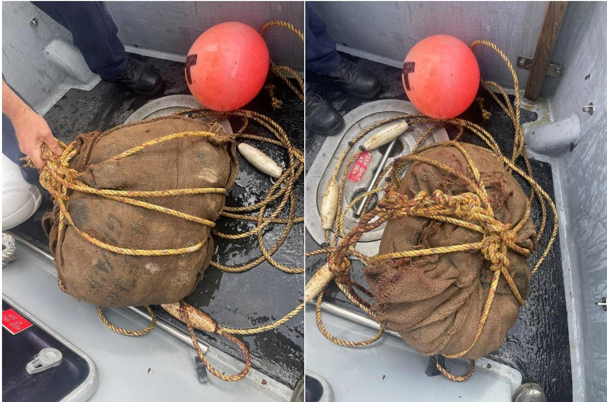
Image 1: Condition of sandbag upon retrieval after 42 days deployment
