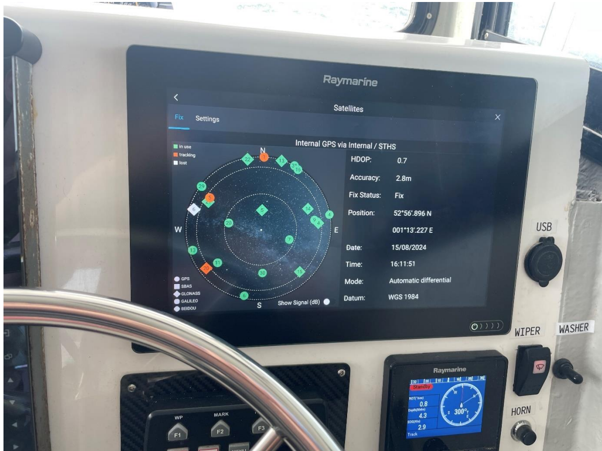
Figure 19: Image showing the DOP reading and accuracy of the vessel GPS on the 15/08/2024 patrol.
