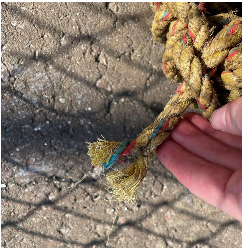
Image 2: Condition of rope which had previously been attached to the marker buoy
